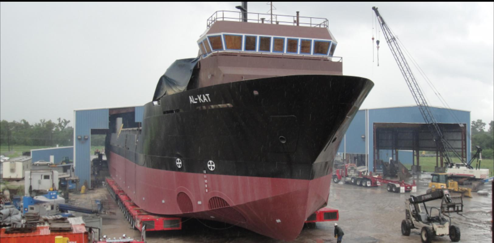
The 1200 ton supply boat was moved using forty lines of SLE spmts with four power pack units. The team moved the vessel from the fabricators shop to the clients drydock for launching. As you can see in the photo, there was a hard rain during the first part of the move, but that didn't stop the team from taking care of business. The spmts were removed once the vessel was on blocks and the drydock submerged. Another day, another workboat successfully moved by the Berard Team!
